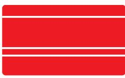
• **Print head dirty or damaged.** Clean or replace the print head.
