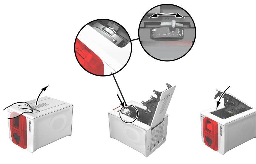
Open the printer cover by pressing on the opening lever, and lifting it up.
