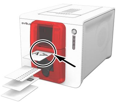
After starting your print task, insert a card into the manual feeder. The card will emerge automatically when printing is complete.
