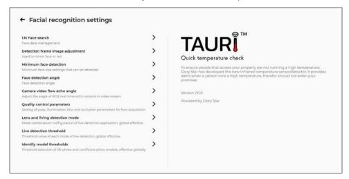
2.5.10 "Detection frame image adjustment" = mirror image shown on screen.
